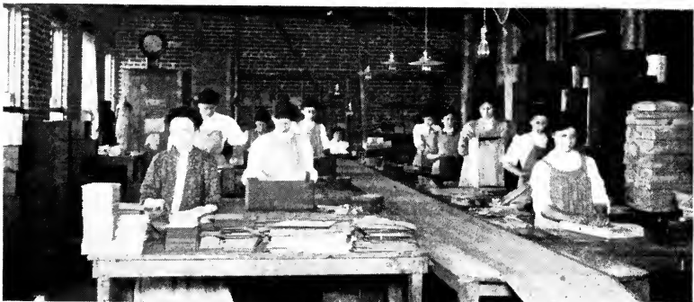
Typical production short cuts are here shown. In making silk bags (above), to contain smokeless powder for the guns of the United States Navy, bottoms and caps are cut out in quantity by an electric blade. Stock for the job in process and for the job next ahead is held in semi-circular racks (middle). A belt-conveyor determines the rate of production in the packing department below
